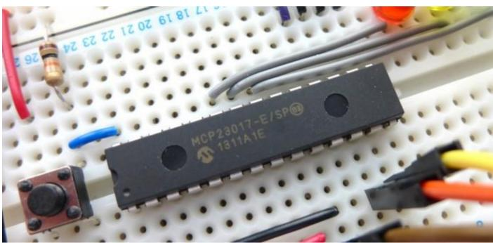
In <u>How To Use A MCP23017 I2C Port Expander With The Raspberry Pi – Part 1</u> I explained how to configure your Pi to use I2C so you could connect an MCP23017 16-bit port expander to it. If you've followed that article and got your circuit ready you are only a few steps away from controlling the chip using a simple Python script.
